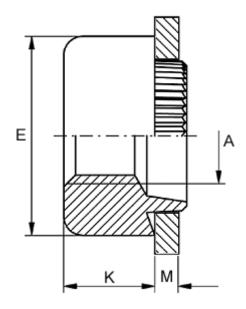
Female thread A = M6Height K = 6.0Outer diameter E = 13.0Plate thickness = 0.9 to 1.0
